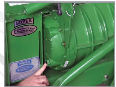
Sight hole for monitoring of oil level in bearing units
