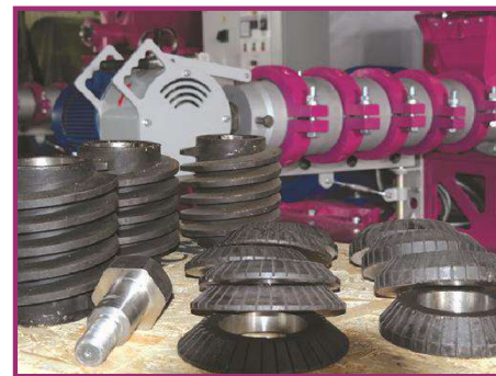
Special wear- resistant reinforcing of screw feeders and milling bowls
