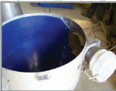
Rhine Liner coating ensures abrasion protection
