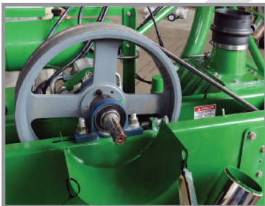
Pneumatic conveyor drive
