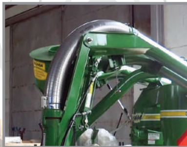
Discharge bar for height adjusting, 360° rotatable
